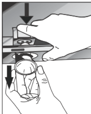
Fig.16: Halogen lamp replacement
